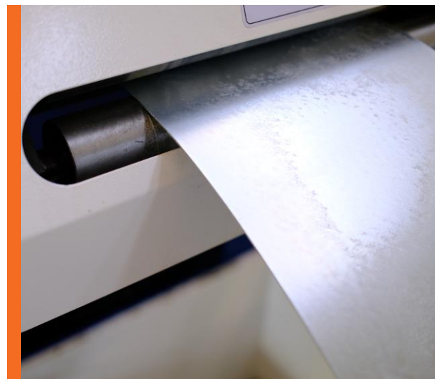
S350-GD (EN10346) steel for LGSF C-profiles
